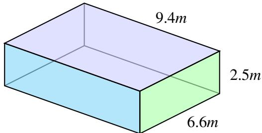
$$V: 6.6 \text{ m} \times 9.4 \times 2.5 \text{ m} = 155.1 \text{ m}^3$$
